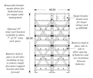
Model shown is IFR516, measurements shown are specifically for the batteries listed on this datasheet, measurements shown in inches
