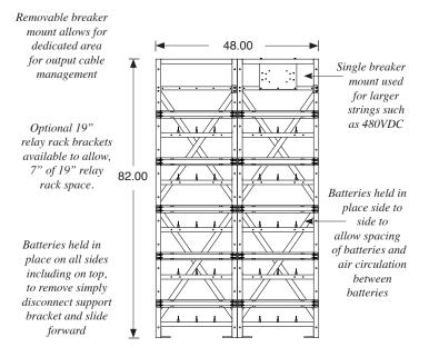
Model shown is IFR512, measurements shown are specifically for the batteries listed on this datasheet, measurements shown in inches Note: Due to the weight of each battery, IntraPack recommends using a lifting device for installing or removing batteries.
