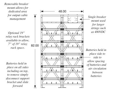
Model shown is IFR512, measurements shown are specifically for the batteries listed on this datasheet, measurements shown in inches
