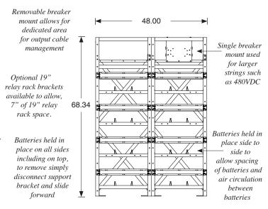
Model shown is IFR416, measurements shown are specifically for the batteries listed on this datasheet, measurements shown in inches Note: Due to the weight of each battery, IntraPack recommends using a lifting device for installing or removing batteries.
