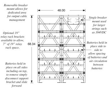
Model shown is IFR412, measurements shown are specifically for the batteries listed on this datasheet, measurements shown in inches Note: Due to the weight of each battery, IntraPack recommends using a lifting device for installing or removing batteries.
