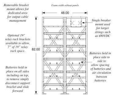
Model shown is IP5F16, measurements shown are specifically for the batteries listed on this datasheet, measurements shown in inches Note: Due to the weight of each battery, IntraPack recommends using a lifting device for installing or removing batteries.
