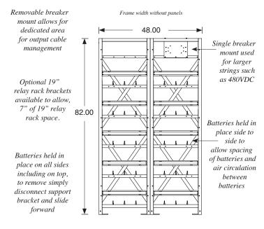
Model shown is IP5F12, measurements shown are specifically for the batteries listed on this datasheet, measurements shown in inches Note: Due to the weight of each battery, IntraPack recommends using a lifting device for installing or removing batteries.
