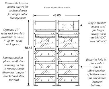
Model shown is IP4F16, measurements shown are specifically for the batteries listed on this datasheet, measurements shown in inches Note: Due to the weight of each battery, IntraPack recommends using a lifting device for installing or removing batteries.
