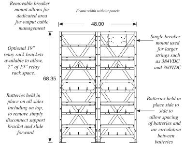
Model shown is IP4F12, measurements shown are specifically for the batteries listed on this datasheet, measurements shown in inches Note: Due to the weight of each battery, IntraPack recommends using a lifting device for installing or removing batteries.
