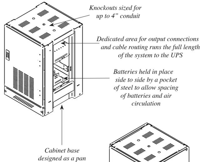
Top view and bottom view shown with panels. Each panel adds .87" to the width
