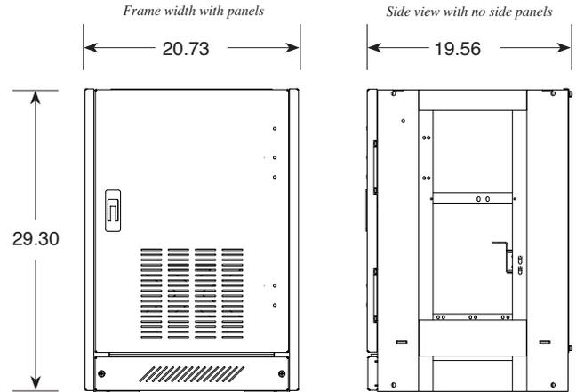
Front view and side view dimensions of frame with panels
